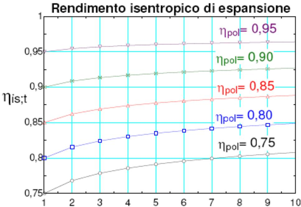
$$\eta_{is,t} = \frac{1 - \beta \left[ - \left( \frac{\gamma - 1}{\gamma} \right) \cdot \eta_{pol,t} \right]}{1 - \beta \left[ - \left( \frac{\gamma - 1}{\gamma} \right) \right]}$$
