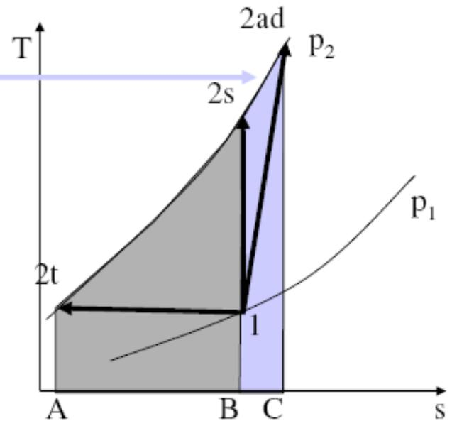
$$W_{ad} - W_s = \frac{\gamma}{\gamma - 1} \cdot RT_1 \cdot \left[ \frac{T_{2ad}}{T_1} - \frac{T_{2s}}{T_1} \right] = \frac{\gamma}{\gamma - 1} \cdot \frac{p_1}{\rho_1} \cdot \left[ \left( \frac{p_2}{p_1} \right)^{\frac{m-1}{m}} - \left( \frac{p_2}{p_1} \right)^{\frac{\gamma-1}{\gamma}} \right]$$
